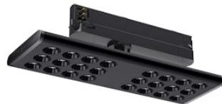
Luminaire for use on a three-phase track. High-quality colour rendering Full Spectrum light source. Also available in The Running Magnet version. This can rotate by 360° on the axis of its rear arm to reach any position relative to the track (from parallel to perpendicular). UGR<19. EN12464 - cd/m<sup>2</sup> @ 65°<3000 compliant.
