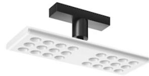
Luminaire for use on The Running Magnet system. High-efficiency light source. This can rotate by 360° on the axis of its rear arm to reach any position relative to the track (from parallel to perpendicular). UGR<19. EN12464 - cd/m² @ 65°<3000 compliant. Casambi, maximum distance between fixtures: 50m.
