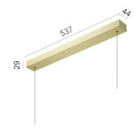
60W – 220/240V power supply included. Kits for Super Line and Super Line Pro Down are equipped with a dip-switch driver to select the maximum intensities.
