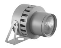
LED source included. Integrated electrical power supply 220-240V ON/OFF. Fixing bracket included. Equipped with a 1000 mm protruding section of neoprene cable and a kit with crimpable connectors and adhesive heat-shrinkable sleeves that guarantee the tightness of the connection. Optional IP68 connectors available. The metal nail for ground installation needs to be ordered separately. Optional accessories to regulate the light beam. Dimmable version available upon request.
