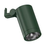
LED COB light source integrated. Integrated electric power supply 220-240 V ON/OFF and adjustable 1-10 V or DALI. Integrated support for pole fixing, for poles with a diameter between 60 and 120 mm and a maximum thickness of 3 mm. Equipped with a 5 m neoprene cable (10 m upon request) for remote connection. To guarantee its water tightness, it is recommended to use flexible cables designed for outdoor use.
