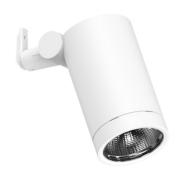
LED COB light source integrated. Integrated electric power supply 220-240 V ON/OFF and adjustable 1-10 V or DALI. Integrated support for pole fixing, for poles with a diameter between 60 and 120 mm and a maximum thickness of 3 mm. Equipped with a 5 m neoprene cable (10 m upon request) for remote connection. To guarantee its water tightness, it is recommended to use flexible cables designed for outdoor use.
