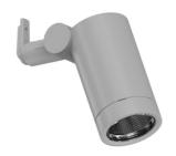
LED COB light source integrated. Integrated electric power supply 220-240 V ON/OFF. Integrated support for pole fixing, for poles with a diameter between 60 and 120 mm and a maximum thickness of 3 mm. Equipped with a 5 m neoprene cable (10 m upon request) for remote connection. To guarantee its water tightness, it is recommended to use flexible cables designed for outdoor use. Upon request: 1-10 V or DALI dimmable version with 24 Vdc remote power supply.
