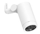
LED COB light source integrated. Integrated electric power supply 220-240 V ON/OFF. Integrated support for pole fixing, for poles with a diameter between 60 and 120 mm and a maximum thickness of 3 mm. Equipped with a 5 m neoprene cable (10 m upon request) for remote connection. To guarantee its water tightness, it is recommended to use flexible cables designed for outdoor use. Upon request: 1-10 V or DALI dimmable version with 24 Vdc remote power supply.
