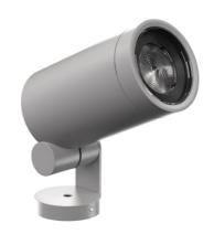
Power LED source included. Equipped with an integrated snoot for higher visual comfort. Collimators are available as an accessory to modify the beam opening. Integrated electric power supply 220-240 V ON/OFF and adjustable 1-10 V or DALI. Minimum L-shaped mounting support integrated. Equipped with a 5 m neoprene cable (10 m upon request) for remote connection. To guarantee its water tightness, it is recommended to use flexible cables designed for outdoor use.
