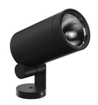
LED COB light source integrated. Integrated electric power supply 220-240 V ON/OFF and adjustable 1-10 V or DALI. Minimum L-shaped mounting support integrated. Equipped with a 5 m neoprene cable (10 m upon request) for remote connection. To guarantee its water tightness, it is recommended to use flexible cables designed for outdoor use.
