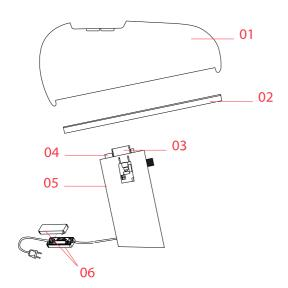
O1. Snoopy Blue reflector RF36696O2. Snoopy glass diffuser RF84656
