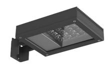
LED source included. Integrated power supply 220-240V ON/OFF and dimmable 1-10V or DALI. Fixing bracket included. Equipped with a M16x1.5 cable guide (for 4.5mm<ø<10mm cables) and IP68 connector. To ensure the tightness of the cable guide it's recommended to use flexible electric cables suitable for exterior use. Optional accessories: protruding arm for walls; feet and arms to install the luminaire on a mast; wall-washer visor and anti-vandalism protection lid. Extraclear transparent glass.
