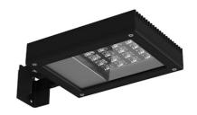
LED source included. Integrated power supply 220-240V ON/OFF and dimmable 1-10V or DALI. Fixing bracket included. Equipped with a M16x1.5 cable guide (for 4.5mm<ø<10mm cables) and IP68 connector. To ensure the tightness of the cable guide it's recommended to use flexible electric cables suitable for exterior use. Optional accessories: protruding arm for walls; feet and arms to install the luminaire on a mast; wall-washer visor and anti-vandalism protection lid. Extraclear transparent glass.
