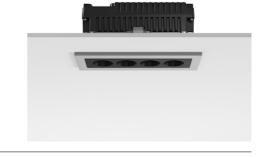
LED light source included. Integrated 220-240V ON/OFF and 1-10V/DALI dimmable electrical power. Equipped with neoprene cable outlet and double cable grommet for in/out connection. Ceiling mounting springs included. Box for brick roofing installation to be ordered separately.
