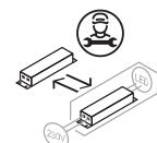
Replaceable control gear by a professional
