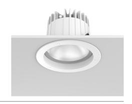
LED source included. Integrated power supply 220-240V ON/OFF and dimmable 1-10V or DALI: remote kit with a 400mm cable section with watertight threaded M12 connector on the luminaire and a 250mm cable section for connection on the mains. This needs to be housed in the junction box for masonry ceilings (it needs to be ordered separately) or set next to the luminaire in case of plasterboard false ceilings. Dimmable version available upon request.
