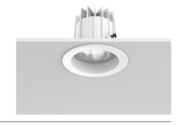
LED source included. Integrated power supply 220-240V ON/OFF and dimmable 1-10V or DALI: remote kit with a 400mm cable section with watertight threaded M12 connector on the luminaire and a 250mm cable section for connection on the mains. This needs to be housed in the junction box for masonry ceilings (it needs to be ordered separately) or set next to the luminaire in case of plasterboard false ceilings. Dimmable version available upon request.
