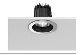
LED source included. Integrated power supply 220-240V ON/OFF and dimmable 1-10V or DALI: remote kit with a 400mm cable section with watertight threaded M12 connector on the luminaire and a 250mm cable section for connection on the mains. This needs to be housed in the junction box for masonry ceilings (it needs to be ordered separately) or set next to the luminaire in case of plasterboard false ceilings. Dimmable version available upon request.
