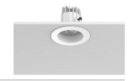
LED source included. Integrated power supply 220-240V ON/OFF and dimmable 1-10V or DALI: remote kit with a 400mm cable section with watertight threaded M12 connector on the luminaire and a 250mm cable section for connection on the mains. This needs to be housed in the junction box for masonry ceilings (it needs to be ordered separately) or set next to the luminaire in case of plasterboard false ceilings. Dimmable version available upon request.
