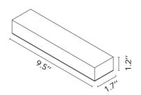
Length: 9.5"; Width: 1.7"; Height: 1.2" Remote class II power supply. UL Listed.
