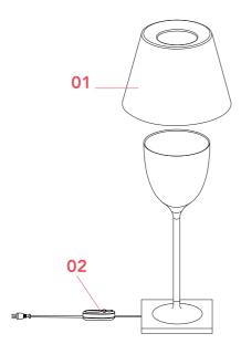
01. Ktribe Floor/Table 2 fumée F6278000 diffuser assembly02. Black Dimmer Switch RF28206
