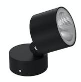
LED source included. LED module configured to work directly on the mains 220-230V ON/OFF. Fixing bracket included. IP68 connector for 6mm<ø<8mm rubber cable. To ensure the tightness of the cable guide it's recommended to use flexible electric cables suitable for exterior use. Ground spike to be ordered separately.
