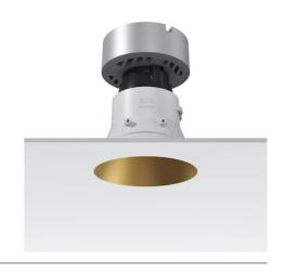
Recessed luminaire with LED light source. Remote transformer not included. Pre-installation frame. To be ordered separately. Diffusing lens included.
