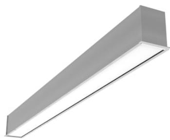
LED modular system for recessed Trim installation, including LED luminaires, aluminum installation profile and diffusers. Drivers included in lighting modules for 220-240V connection to mains or to other lighting modules.
