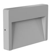
LED source included. Remote electrical power supply 24V dc to be ordered separately. Equipped with a 300 mm protruding section of neoprene cable and a kit with crimpable connectors and adhesive heat-shrinkable sleeves that guarantee the tightness of the connection. Optional accessories: satin aluminum reflector to increase the luminous flux; 500mm tall, extruded post for the bollard version. Anchor plate to be recessed with mortar needs to be ordered separately. Dimmable.
