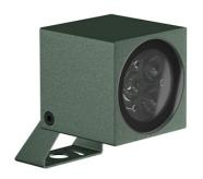
LED source included. Electric remote 24V dc ON/OFF power supply to be ordered separately. Wall fixing bracket included. The luminaire is equipped with a protruding, neoprene, 250 mm cable and a wiring kit with crimp connectors and adhesive heat-shrink tubing guaranteeing the water tightness of the connection. Extra clear transparent glass.
