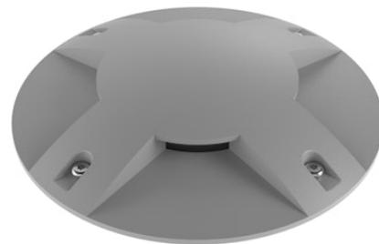
LED light source included. Integrated electric power supply 220-240V ON/OFF. Requires a junction box to be ordered separately. The luminaire is equipped with a protruding, neoprene, 400 mm cable with an M12 watertight screw-on connector towards the luminaire, and with a 300 mm cable for the connection to the power line. Adjustable light intensity version available upon request.
