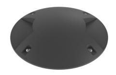
LED source included. 24V dc remote electric power supply to be ordered separately. Requires a junction box to be ordered separately. The luminaire is equipped with protruding, 250 mm cable with an M12 watertight screw-on connector. Optional accessories: 5000 mm cable and 300 mm splitter cable with M12 connectors for multiple installations.
