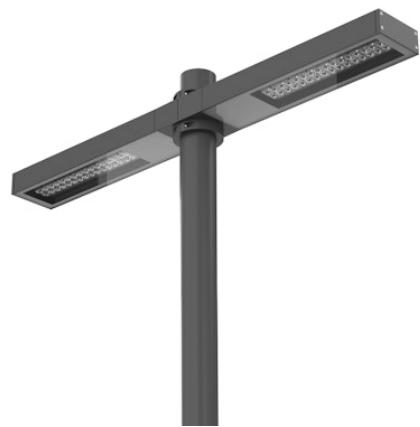
LED source included. Integrated power supply 220-240V ON/OFF and dimmable 1-10V or DALI. Fixing bracket included. Equipped with a 400mm protruding neoprene cable section and IP68 connectors. Double socket for 102mm diameter post. The post must be ordered separately. Smart-City version available upon request.
