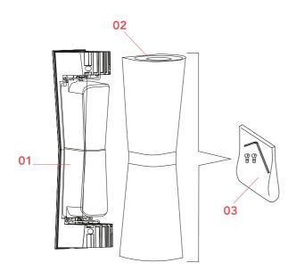
01. Clessidra Wall attachment and F1582030 internal lamp body 40°+40°
