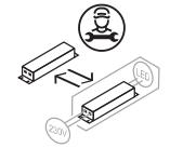
Replaceable control gear by a professional
