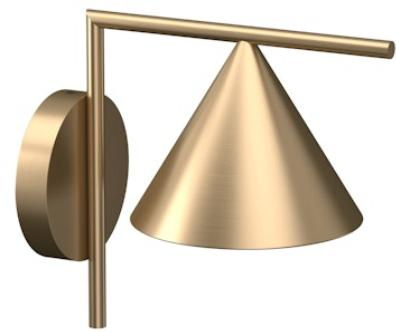
Luminaire for wall-mounting with diffuse light emission and fixed head. LED light source included. Integrated 220-240V ON/OFF or 1-10V/DALI dimmable electrical power. Connection is quickly ensured in the rose with the plug & play electrical connection and the IP68 connector included. Clamp bracket included. 110V version upon request.
