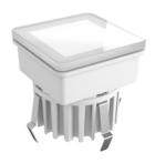
LED source included. 24V dc remote electric power supply to be ordered separately. Requires a junction box to be ordered separately. The luminaire is equipped with a protruding, neoprene, 200 mm cable with an integrated H2O STOP connection system and a wiring kit with crimp connectors and adhesive heat-shrink tubing guaranteeing the water tightness of the connection. Glass with opal diffuser. Adjustable light intensity.
