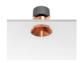
LED luminaire for recessed mounting into plasterboard ceilings. Once installed, the luminaire edge projects from of the ceiling 0.39" creating a unique and very refined aesthetic effect. The luminaire's body is injection molded aluminium. It is available in three sizes: Bon Jour 45 (Ø 1.77"), 90 (Ø 3.54") and 145 (Ø 5.71"). Reflector made of anodized gloss aluminium with diffuser element made of polycarbonate.
