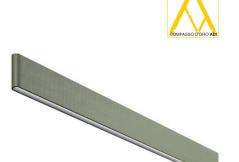
'Electromechanical profile for interior use with integrated linear lighting for suspended installation available with 78.75" or 118.12" lengths. Installation via suspension leather or fabric straps on the ceiling and remote power kit, to be ordered separately. Up&Down system controlled via DALI or CASAMBI individually and via 1-10V all together (Broadcast).
