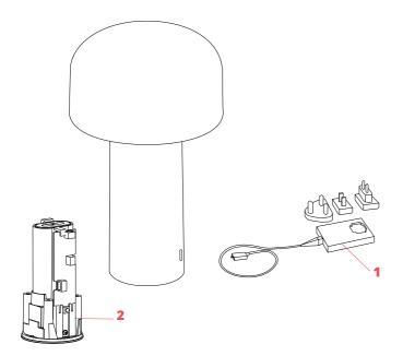
O1. Power charger with electrical RF1035109 cable & plugs
