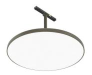
General lighting LED module to be installed in the Zero Track system. Incorporated DC/DC electronic converter. Module regulated via 0/1-10V DALI or Casambi driver in broadcast mode. Dimmer not included. To individually control the lights, select integrated Casambi versions. Not suitable for vertical installations.
