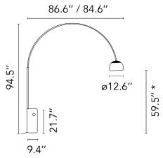
\*The diffuser can be adjusted to 67" or 72.8".
