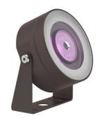
RGB LED source included. Remote electrical power supply with DMX 3chx350mA interface to be ordered separately. Serial connection. Equipped with a 2000 mm protruding section of neoprene cable and a kit with crimpable connectors and adhesive heat-shrinkable sleeves that guarantee the tightness of the connection. Transparent screen-printed glass. The metal nail for ground installation needs to be ordered separately.
