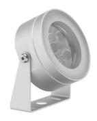
LED source included. Remote electrical power supply 24V dc ON/OFF to be ordered separately. Parallel connection. Equipped with a 2000 mm protruding section of neoprene cable and a kit with crimpable connectors and adhesive heat-shrinkable sleeves that guarantee the tightness of the connection. Fixing bracket included. Extraclear transparent glass. The metal nail for ground installation needs to be ordered separately.
