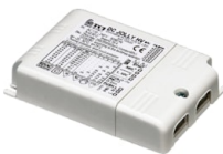
OPTIONAL Power supply FA129 Power supply 16 x 1W/ 110÷240V - Iout 350mA (12x1W@110V) IP20 Class II Selv Eq. Dimmable Push-Dimm Or 1.10V
