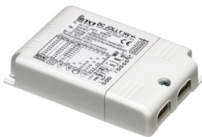
OPTIONAL Power supply FA129 Power supply 16 x 1W/ 110÷240V - Iout 350mA (12x1W@110V) IP20 Class II Selv Eq. Dimmable Push-Dimm Or 1.10V
