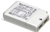
OPTIONAL Power supply FA135 Power supply 13 x 2W/ 110÷240V - Iout 500mA (7x2W@110V) IP20 Class II Selv. Eq. Dimmable Push-Dimm Or 1.10V
