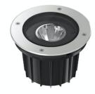
LED light source included. Integrated 24V dc ON/OFF remote electric power supply. Adjustment on vertical axis: 15° max. Rotation on horizontal axis: 359° max. Remote power supply that must be placed in a junction box, equipped with a protruding, 400 mm cable with an M12 screw-on connector that guarantees the water tightness of the luminaire, and with a 250 mm cable for the connection to the power line. Extra clear transparent glass. Adjustable light intensity version available upon request.
