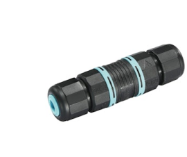
OPTIONAL Accessory F990C00A000 2 way terminal block 4 poles IP68 H2O stop. (ø5,5÷12mm cable)
