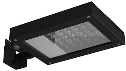
LED source included. Integrated power supply 220-240V. Graduated fixing bracket included. Equipped with a M20x1.5 cable guide (for 7mm<ø<13mm cables) and IP68 connector. To ensure the tightness of the cable guide it's recommended to use flexible electric cables suitable for exterior use. Optional accessories: protruding arm for walls; feet and arms to install the luminaire on a mast; wall-washer visor and anti-vandalism protection lid. Extraclear transparent glass.
