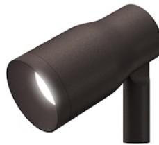
Spot adjustable head for installation on ground poles or on wall base. Poles and base to be ordered as separated accessories. Heads are equipped with a dismountable ferrule, to insert flood lens or up to two honeycombs, (to be ordered as separate accessories). 24V remote power supply to be ordered separately. Each head comes with a 2000 mm lenght outgoing cable and a wiring kit.
