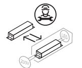
Replaceable control gear by a professional
