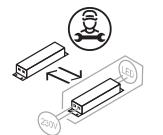
Replaceable control gear by a professional
