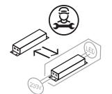
Replaceable control gear by a professional
