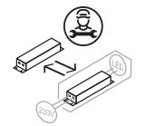
Replaceable control gear by a professional
