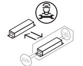
Replaceable control gear by a professional
